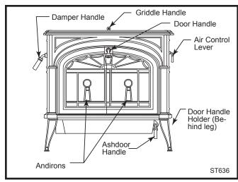
Fig. 18 The Encore controls are conveniently located and easy to operate.
